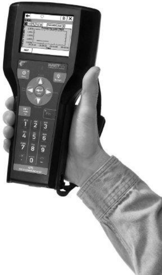
Figure 3-4. Hand-held Device to Check and Set Transmitter Calibration
